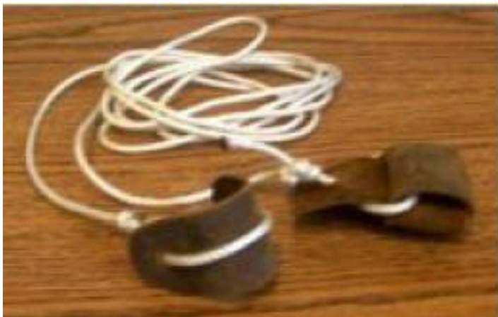
Figure 3: A completed bow stringer
